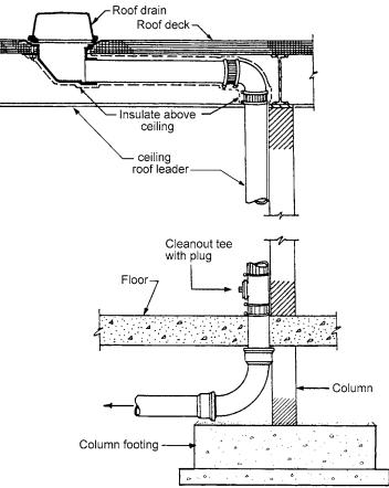
Figure 4-8 Typical Roof Drain and Roof Leader Source: Reprinted, by permission, from *Cast Iron Soil Pipe and Fittings Engineering Manual* (Cast Iron Soil Pipe Institute, 1976)
