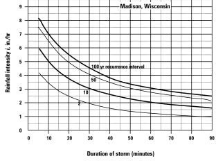
Figure 4-3 Intensity-Duration-Frequency Curve
