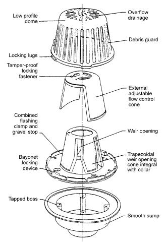
Figure 4-9 Example of a Controlled-flow Drain Source: Reprinted, by permission, from the Jay R. Smith catalog
