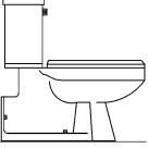
Figure 1-3 Floor-Mounted, Back-Outlet Water Closet
