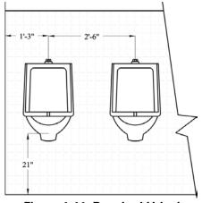
Figure 1-11 Required Urinal Spacing
