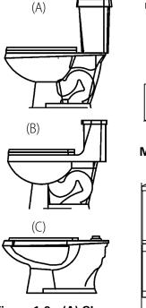
Figure 1-2 (A) Close-Coupled, (B) One-Piece, and (C) Flushometer Water Closets
