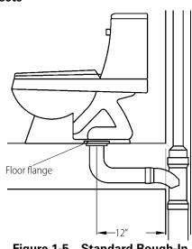
Figure 1-5 Standard Rough-In Dimension for a Water Closet Outlet to the Back Wall
