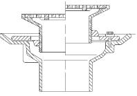
Figure 1-20 Floor Drain
