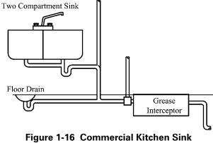
Figure 1-16 Commercial Kitchen Sink Discharging to a Grease Interceptor
