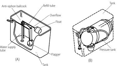
Figure 1-8 (A) Gravity Tank and (B) Flushometer Tank
