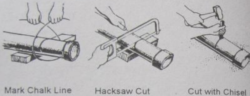
FIGURE 3-8 CUTTING CAST IRON PIPE
