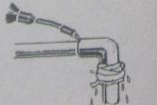
Wrap Soldered Joint with Wet Rags
