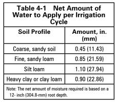
A sufficient amount of water must be applied during each irrigation period to ensure penetration to the root zone. Table 4-1 suggests guidelines for several soil profiles (the net amount of water to apply per irrigation cycle). In the absence of any specific information on the soil and local weather conditions, the irrigation system may be designed for  $1\frac{1}{2}$  inches (38.1 mm) of water per week.
