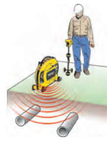
Induce a signal to locate utilities.
